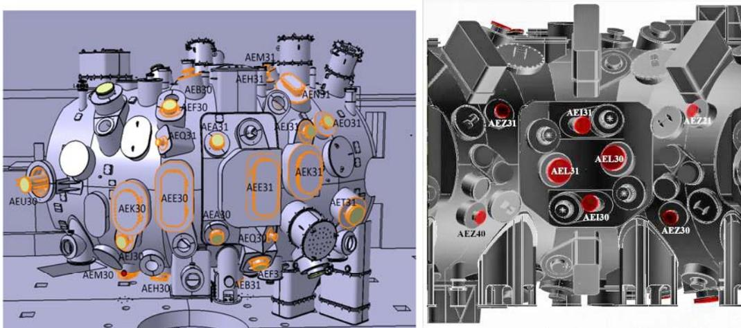
Fig. 1: Diagnostics ports in half modules 30 & 31:
