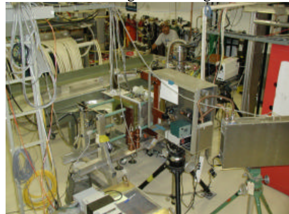
Figure 3: A photo of the new FRX-L laboratory (9/2001), with the FRX-L FRC in the middle of the photo, partially hidden in the foreground by the 3.39 micron laser interferometer, and in the background by the fan-shaped parallel-plate header which feeds currents to the 1-turn theta-coils.
