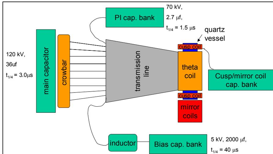
Fig. 2. Simplified experimental schematic of the FRX-L device.
