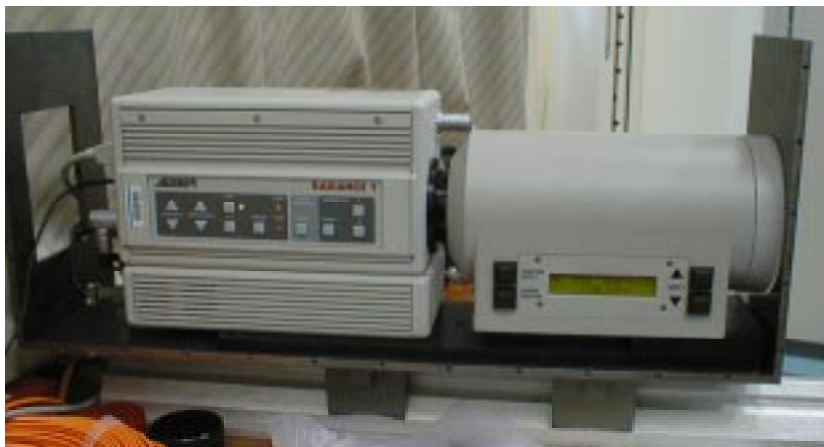
Figure 1: Side view of Amber IR video camera, 250 mm Ge/Si lens, with soft-iron shield box partly removed.
