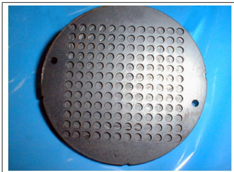
**Figure 4:** 12 x 12 copper mask, with gold foil which has been blackened with graphite spray.
