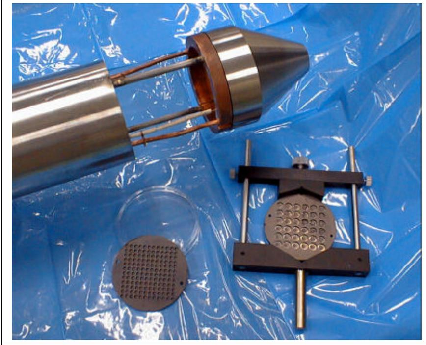
**Figure 3:** Front assembly of LHD imaging bolometer prototype, with two mask/foil assemblies shown. A mask/foil assembly is placed at the back of the water-cooled pinhole camera nosecone. Two (copper-constantan) thermocouples, and tubes carrying water, are also attached to the copper housing.
