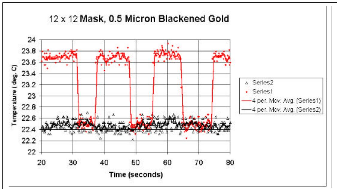
**Figure 6:** Point temperature measurement made by Agema 9600 IR camera of a foil pixel being illuminated by a 1.5 mW calibration laser (in air).
