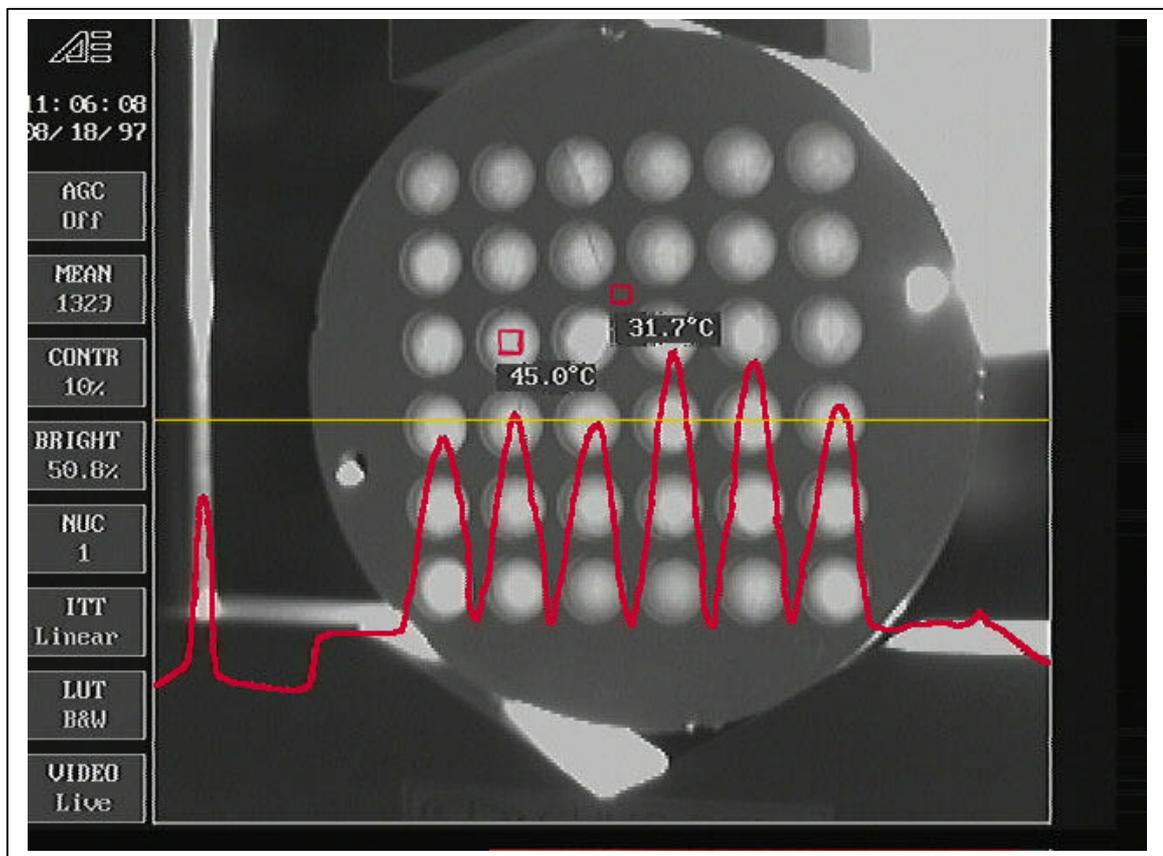
**Figure 8:** Heating of a masked 6x6 foil in air caused by a 100 watt heat lamp, 20 cm away from the mask, is easily seen by the Amber IR Video camera. The IR intensity profile on a line across the middle of the image, is graphically displayed near the bottom of the image. The temperature near the edge of each pixel is clamped by the thermal inertia of the thick copper mask.
